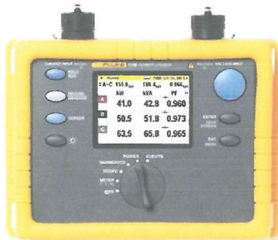
Fig. 3.1 FLUKE 1735 Power Logger.
